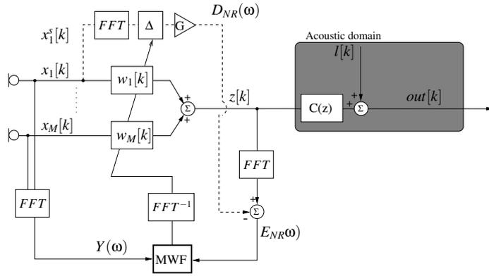
Figure 1: MWF-based NR in hearing aids framework
